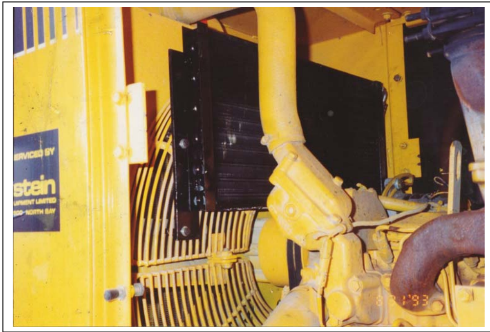
Condenser mounted in place. May not me exactly as shown.
